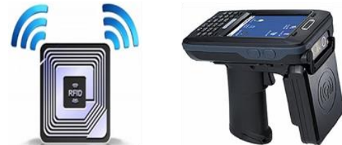
Figure 2.4. RFID chip and portable RFID reader
