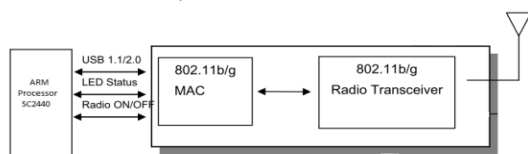
Fig. 5 The interface block diagram of Wi-Fi transmitter
